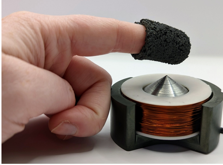
Figure 3.1: The fingertip actuation device, consisting of a wearable magnetic fingertip sheath and an external electromagnet.
